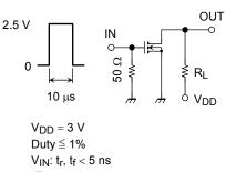
$\begin{array}{l} \text{Duty} \geqq 1\% \\ \text{V}_{\text{IN}} : t_r, \, t_f < 5 \, \text{ns} \\ (\text{Z}_{\text{out}} = 50 \, \Omega) \\ \text{Common Source} \\ \text{Ta} = 25^{\circ}\text{C} \end{array}$
